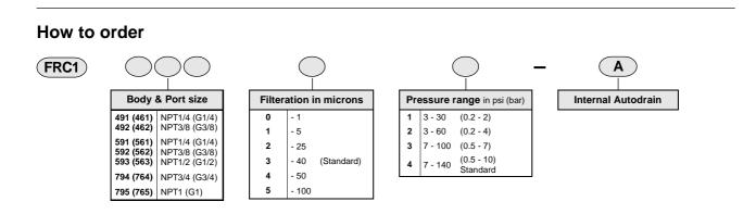
Ordering example :- Filter Regulator Combination - 3/8 size (with NPT 3/8 (G3/8) port) with a 5 microns Filter, pressure range 7 - 100 psi with Internal Autodrain: Ordering No: FRC1492 (1462) 13 - A.
