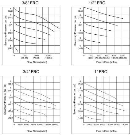
Flow graphs are for 40µm filterations only
